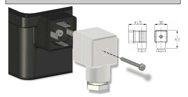
Our cable glands are designed for cables with a diameter between 7mm and 12mm.
