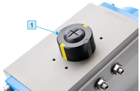
Fig. 3-13 Operating and display elements of the rotary actuator bar-acturn Longitudinal design = open position Transverse design = closed position
