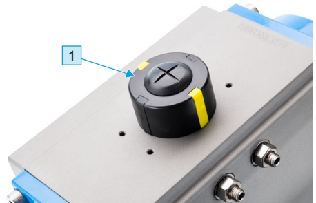
Fig. 3-12 Operating and display elements of the rotary actuator bar-acturn Longitudinal design = closed position Transverse design = open position
